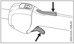
Press down the throttle trigger lockout and open the throttle – the choke knob moves to the run position I. After a cold start, warm up the engine by opening the throttle several times.
