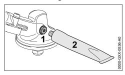
Check grease level after every 25 hours of operation and re-lubricate if necessary.
