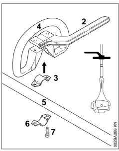
Place the clamp (3) in the loop handle (4) and position them both against the drive tube (5).
