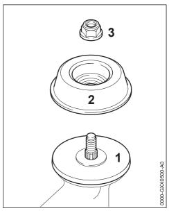
Depending on the cutting attachment, it may be necessary to use the nut (3) and rider plate (2). The thrust plate (1) must be used with all cutting attachments.
