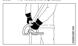
For versions with loop handle and loop handle with barrier bar, left hand on the loop handle, right hand on the control handle – even if you are left-handed
