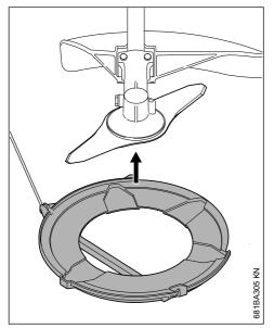
Fit the transport guard on the cutting attachment from below.
