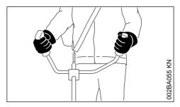
Right hand on control handle, left hand on grip on handlebar.
