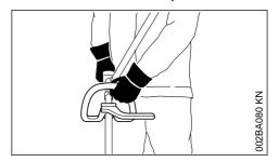
For versions with loop handle and loop handle with barrier bar, left hand on the loop handle, right hand on the control handle – even if you are left-handed
