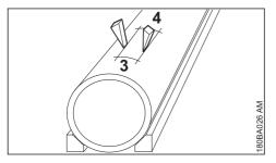
If the severed part remains in the recess after cutting (due to wedges, ridges used), do not make any further cuts – break the severed part
