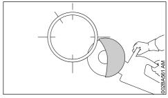
Use the upper quarter of the abrasive wheel for cutting the opposite lower side.
