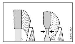
Do not cut into the base course (frequently chipped stones and gravel) when cutting roadway pavement – cutting in chipped stones and gravel is revealed by light-colored dust – excessive undercut may occur as a result – **Danger of shattering!**
