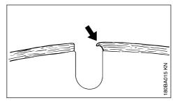
If work continues with dull segments, these may soften due to the high heat generated – the parent wheel is annealed and its strength is compromised – this can lead to stresses that are clearly recognizable by gyrations of the abrasive wheel. Do not continue to use the abrasive wheel
