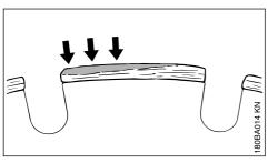
Built-up edges take the form of a light gray deposit on the tops of the diamond segments. This deposit on the segments clogs the diamonds and blunts the segments.
