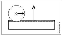
Grind a guide groove (A) along the line marked
