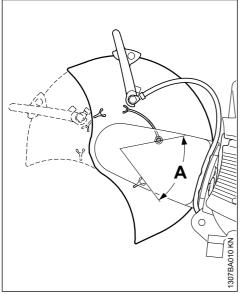
Rotate the guard forwards and backwards as far as possible – adjustment range (A) must be limited by the stop pin
