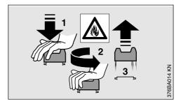
Never use a tool to open or close the bayonettype fuel cap. This could damage the cap and cause fuel to leak out.
