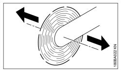
When a cut-off machine with an abrasive cutting wheel rotating is moved in the direction of the arrow, a force is produced which causes the machine to tip sideways.
