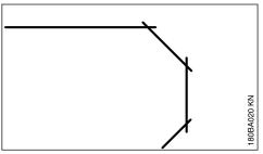
Make curves in multiple operations – make certain that the abrasive wheel does not tilt
