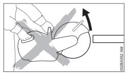
If possible, avoid using the upper quarter of the abrasive cutting wheel for cutting. Use extreme caution when guiding the abrasive cutting wheel into a cut, do not twist or push into the cut
