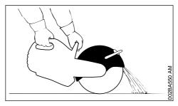
Set the abrasive cutting wheel guard correctly: Guide particles of material away from the user and machine.
