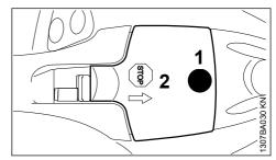
Unscrew screw (1) and remove cap (2) – screw (1) is secured in the cap (2) to prevent loss
