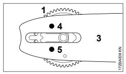
Position the tensioning gear (1) against the guide bar (3) so that the stud (4) projects through the upper hole and the short guide peg (5) locates in the lower hole.
