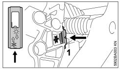
► Place the shutter with the opening in the direction of the chain saw (winter operation) – arrow points toward symbol \* – shutter must audibly snap into place
