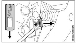
► Using the combination wrench or a screwdriver, pry the shutter out of the ☆ (summer operation) position
