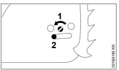
► Turn the screw (1) counterclockwise until the tensioner slide (2) butts against the left end of the housing slot.
