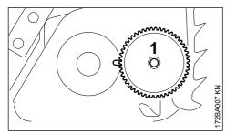
Remove the tensioning gear (1) and turn it over.
