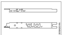
STIHL filing gauge (special accessory, see table "Sharpening tools") – a universal tool for check-
