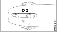
Screw the nut (2) on to the stud as far as stop by hand.
