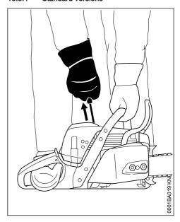
► With the right hand, pull the starter grip slowly until you feel it engage – and then give it a brisk strong pull – simultaneously press down on the handlebar – do not pull the starter rope out all the way – risk of breakage! Do not let the starter grip snap back – guide it vertically back into the housing so that the starter rope can rewind properly
