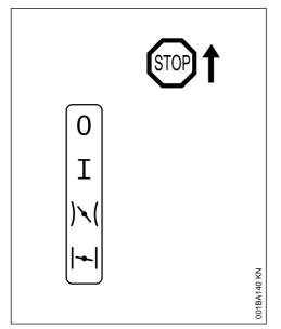
Stop 0 - engine off - ignition is switched off
