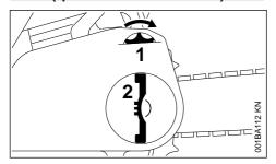
Retensioning during cutting work:
