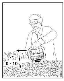
Hold the cutter bar at an angle of 0° to 10° as you swing the hedge trimmer horizontally.
