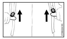
• Lift the tabs of the sliding adjusters.
