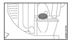
Before fueling, clean the filler cap and the area around it to ensure that no dirt falls into the tank.
