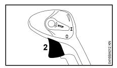
Blip the throttle trigger – the choke knob automatically returns to "I"
