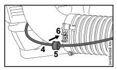
• Engage the throttle cable (4) with sleeve (5) in the hose clamp (6).
