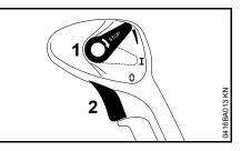
The throttle trigger (2) can be locked in any position.
